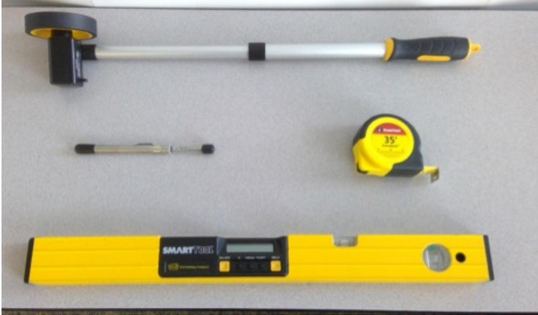
*These tools are used by a surveying team to measure sidewalk slope, door pressure and other accessibility issues.*
